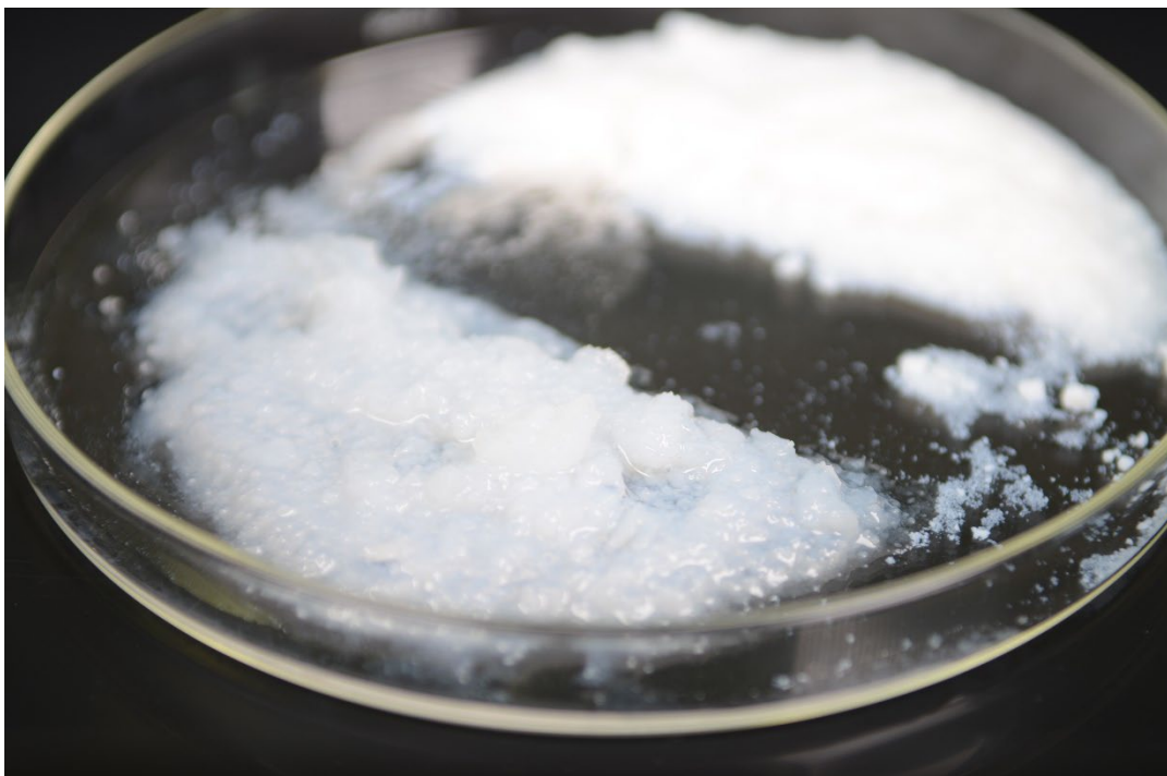
Silicon increases the water-holding capacity of the soil: like a sponge, amorphous silicate attracts water molecules, which accumulate in a gel shell around the silicate core, as can be seen here in the picture. Source: © Hendrik Schneider / ZALF | Picture in color and print quality: http://www.zalf.de/de/aktuelles
