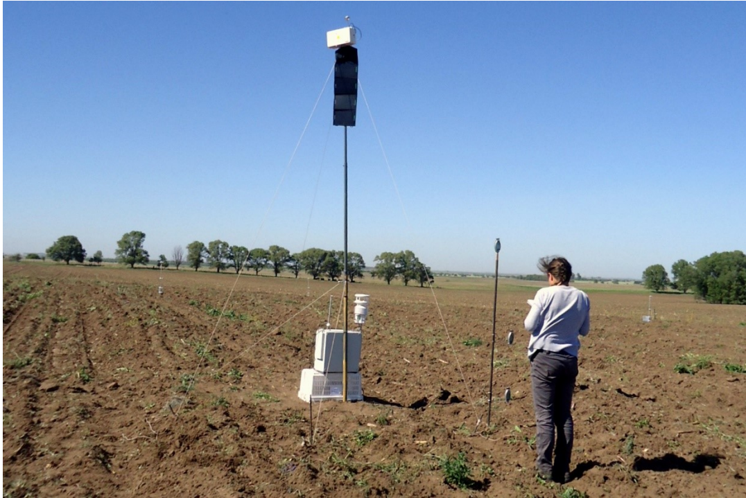
Caption: Field instruments for the analysis of wind erosion and dust emissions | Source: © ZALF / Roger Funk | Image source in color and print quality: http://www.zalf.de/de/aktuelles/meldungen_alle
