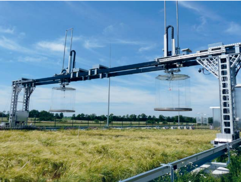
Mobile gantry crane system to monitor flux rates of CO 2 , CH 4 , and N 2 O at the long-term field experiment CARBOZALF (AgroScapeLab Quillow)
