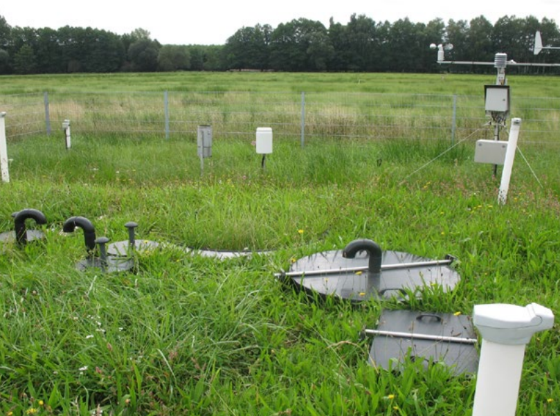
Groundwater lysimeter station in Spreewald wetland, © Ottfried Dietrich | ZALF
