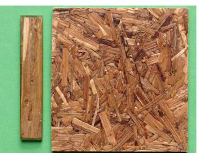
Material samples for demonstration purposes and stability tests made of alfalfa stems and linseed oil-based epoxy resin, manufactured by Bio-Composites and More GmbH (B. A. M.).
