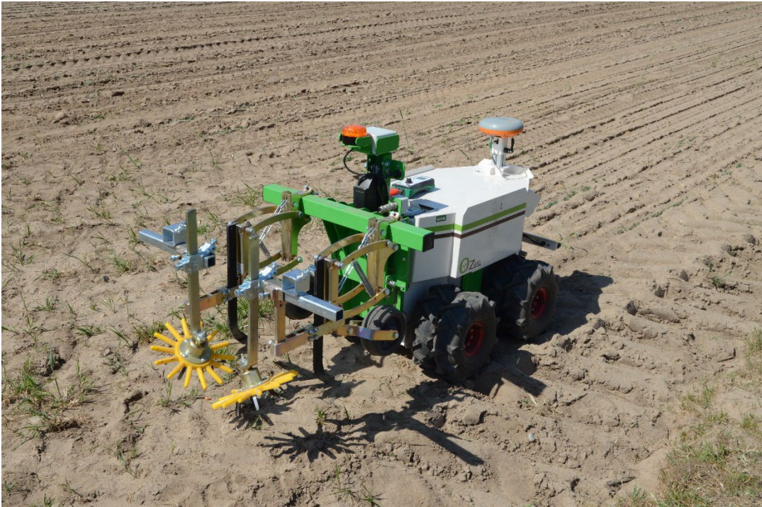
Starting this year, the team of the "patchCROP" landscape laboratory has been working with an agricultural robot to manage the land, for example to control weeds. Source: © Sibylle Krickel / ZALF | Image source in color and print quality: http://www.zalf.de/de/aktuelles
