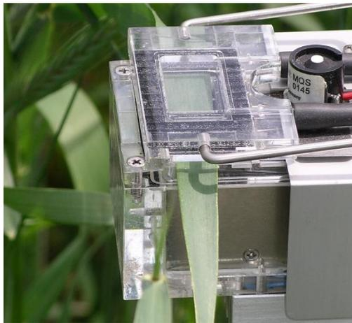
cuvette. However, comparability of such measurements requires that they are carried out under strictly standardised conditions. Influencing factors such as photosynthetically active radiation (PhAR), temperature and relative humidity or air-to-leaf vapour pressure deficit (ALVPD) must be able to be kept constant in the measuring cuvette. The existing instrument (LCproT, ADC, Hoddesdon, UK) offers these possibilities. The aim of this research is to investigate
