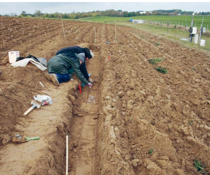
Tracer application (KBr) underneath a cultivated topsoil along a 10 m trench perpendicular to the slope above plot LP7 of the CARBOZALF-D experimental field
