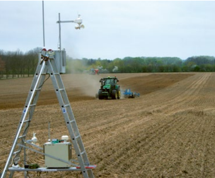
Measurement of dust emissions during tillage directly after manure application
