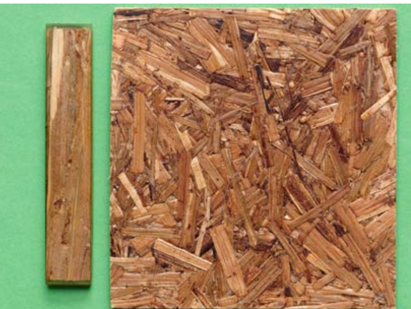
Material samples for demonstration purposes and stability tests made of alfalfa stems and linseed oil-based epoxy resin, manufactured by Bio-Composites and More GmbH (B.A.M.).
