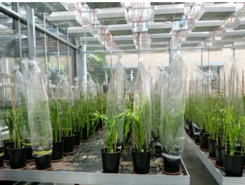
Pot experiment at the project partner IPK Gatersleben within the VOLCORN consortium using common wheat ( Triticum aestivum L.). Individual plants were hermetically isolated in order to measure VOC emissions.
